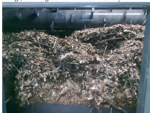
A disintegrator roll breaks possible blocks of frozen fuel.
