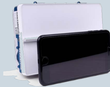
Echodyne phased array RADAR
