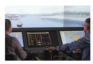
Safety validation of autonomous navigation systems using a ship handling simulator
