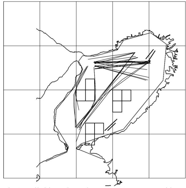
Fig.4.5 All ship's planned route at 18:00-21:00 with avoid towing ship area
