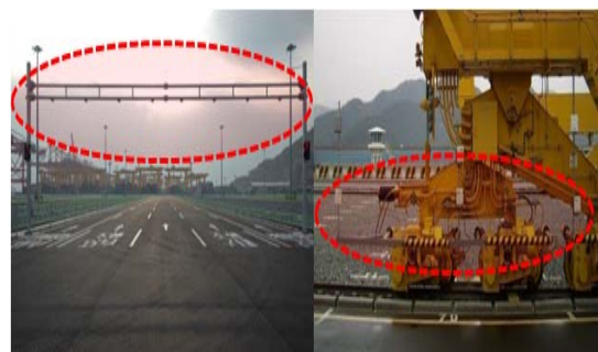
<Fig. 6> RFID based external truck interface (Installed form)
