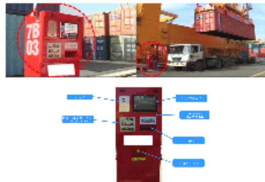
<Fig. 5> Kiosk based external truck interface (Actually operated)
